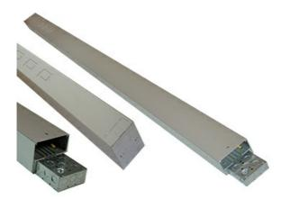
Two-compartment large capacity pole. Furnished unwired without outlets. Box ended with industry sized knockouts. Standard heights: 10' 2" (3.1m) (NP800C-10-2B), 12' 8" 3.9m) (NP800C-12-8B), 15' 2" (4.6m) (NP800C-15-2B)
