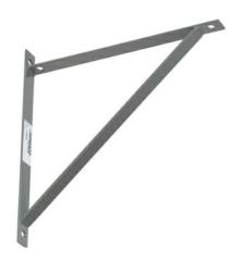
Shelf brackets attach to the wall and extend up to 24 in for heavy duty runway support. Runway is secured to the bracket with J-bolts (included). Made of 3/16 in x 1 in, steel bar. Hardware is zinc plated and dichromated.
