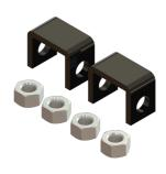
Use closed clips with 1-1/2 in stringers to secure runway to threaded rods when suspending runway from the ceiling. Also use when stacking runway. Use with 5/8 in-11 in threaded rod. Made of 1/4 in x 1-1/2 in steel bar. UL classified.
