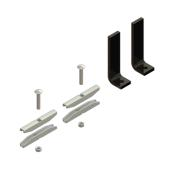
Cable runway feet anchor runway to the wall or floor. Feet are attached to runway with clamps. Made of 3/8 in x 1-.5 in, steel bar. Kit includes two 6 in. cable feet, four straight clamps, two 3/8-16 x 2.25 in carriage bolt, and two 3/8-16 hex nut.
