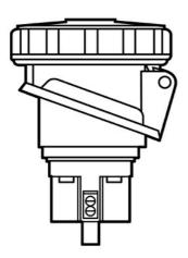
Triple-Pole, 4-Wire, Pin and Sleeve Receptacle. 100A, 3/480V.
