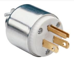
Armor Plug Grounding in white with two poles and three wires. Its rugged nylon construction provides impact and chemical resistance. All 3-wire terminals are located on the same plane, allowing for quick wire termination from any angle. 15A, 125V.
