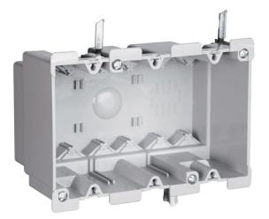
Triple Gang, Old Work Switch and Outlet Box with Swing-Bracket for mounting. Adjusts from 1 1/4-inch down to 1/8-inch. Six Auto/Clamps for Each End. 10 pack.
