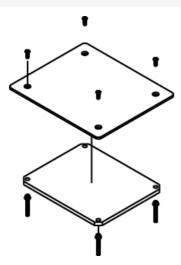
Aluminum top plate with steel support plate and four (4) adjusting screws.
