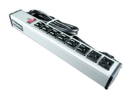
Eight outlets, rugged gray aluminum housing, 15A, lighted switch. 6' (1.8m) 14/3 SJT black cord with NEMA5-15 plug. Length 15" (381mm). Receptacle center-to-center 1 1/4" (32mm). Snap-on, slide-off mounting.
