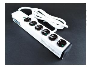
Six outlets. Rugged white aluminum housing. 6' (1.8m) 14/3 SJT white cord with NEMA5-15 plug. Length 13 1/4'' (337mm). Receptacle center-to-center 1 1/2'' (38mm). Snap-on, slide-off mounting. Not for use in critical care enviornments. NOTE: Not for use where Article 517 of NEC requires Hospital Grade Outlets.
