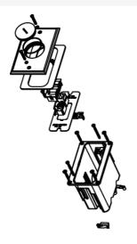
Includes single-gang box, device plate with two openings for communication devices, and brass cover with one screw plug. For hole cut dimensions, see installation instructions sheet. Box Dimensions: 2 1/8" W x 3 3/4" L x 3 7/8" D (54mm W x 95mm L x 98mm D) Device Plate: 3 1/8" W x 4 15/16" L (79mm W x 125mm L).
