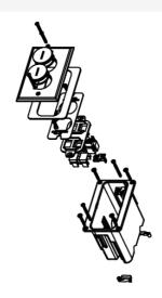
Includes single-gang box, 106 adapter with four openings for communication devices, and nickel cover with two screw plugs. For hole cut dimensions, see installation instructions sheet. Box Dimensions: 2 1/8" W x 3 3/4" L x 3 7/8" D [54mm W x 95mm L x 98mm D] Device Plate: 3 1/8" W x 4 15/16" L [79mm W x 125mm L].
