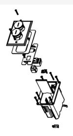
Includes single-gang box, divider, one 15A, 125V receptacle, one opening for communication device, and brass cover with two screw plugs. For hole cut dimensions, see installation instructions sheet. Box Dimensions: 2 1/8" W x 3 3/4" L x 3 7/8" D (54mm W x 95mm L x 98mm D) Device Plate: 3 1/8" W x 4 15/16" L (79mm W x 125mm L).
