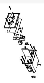
Includes single-gang box, divider, one 15A, 125V receptacle, one opening for communication device, and nickel cover with two screw plugs. For hole cut dimensions, see installation instructions sheet. Box Dimensions:  $2\ 1/8$ " W x  $3\ 3/4$ " L x  $3\ 7/8$ " D (54mm W x 95mm L x 98mm D) Device Plate:  $3\ 1/8$ " W x  $4\ 15/16$ " L (79mm W x 125mm L).
