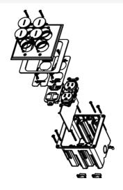
Includes dual-gang box, one 15A tamper-resistant duplex receptacle, 106 adapter with four openings for communication devices, and nickel cover with four screw plugs. For hole cut dimensions, see installation instructions sheet. Box Dimensions: 3 1/4" W x 3 3/4" L x 3 7/8" D (83mm W x 95mm L x 98mm D) Device Plate: 4 7/8" W x 5 1/16" L (124mm W x 129mm L).
