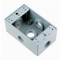
Weatherproof 1 Gang Box, 5 Hole 1/2"", 17.0 Cu.In.,Gray (1 Hole Each End, 1 Hole Each Side, 1 Hole in Back)
