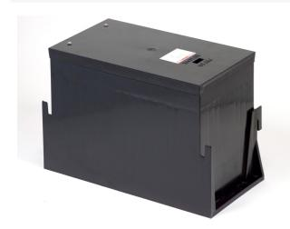
The single service 2-gang Outdoor Ground Box is made from a UV rated nonmetallic material and has been designed to withstand the harsh outdoor environments. The box can accept up to (2) 1 1/4" trade size PVC conduit feeds. Boxes are designed to be installed separately or ganged together, for greater capacity and flexibility. They work with XB814 cover assemblies (sold separately).
