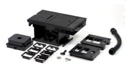
The black Outdoor Ground Box low voltage cover assembly is designed to accept up to 12 communication ports and 8 Legrand AVIP devices. NOTE: Cover must be closed while in use. Use only cables that are rated for outdoor use.NOTE: Maximum length of connector allowed at end of cable is 2" [51mm].
